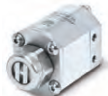
AA10000AUH-104210 Rear liquid inlet Typical flow range: 0.0017 - 0.47 gpm (0.006 - 1.8 lpm) Stainless steel, Viton or EPDM seals, PPS and PEEK Up to 15,000 cycles per min Side liquid inlet version for low profile mounting also available
