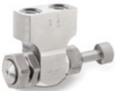
1/4JACN – Air and liquid inlets on the same side of the nozzle body – 90° to spray direction – with manual shut-off needle
