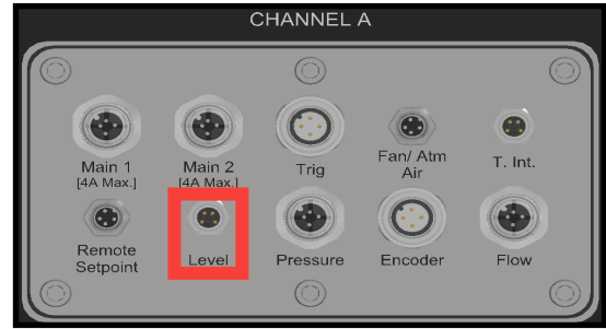
Plug and Spray connections, level sensor
